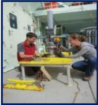
Hydro-Geologist rigging up a flow meter
